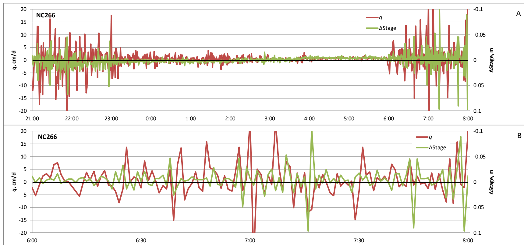
Figure 35. Seepage in centimeters per day (cm/d) and change in stage ( \Delta Stage), in meters (m), at NC266. Chart A shows the 1-minute values of seepage and \Delta Stage on June 15–16, 2017. Chart B shows the 1-minute values of seepage and \Delta Stage on June 16, 2017, from 06:00 to 08:00. The right axes are plotted inversely.
