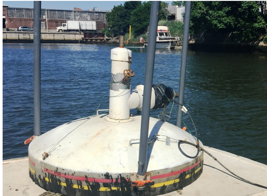
Photo of electromagnetic seepage meter on boat deck.
