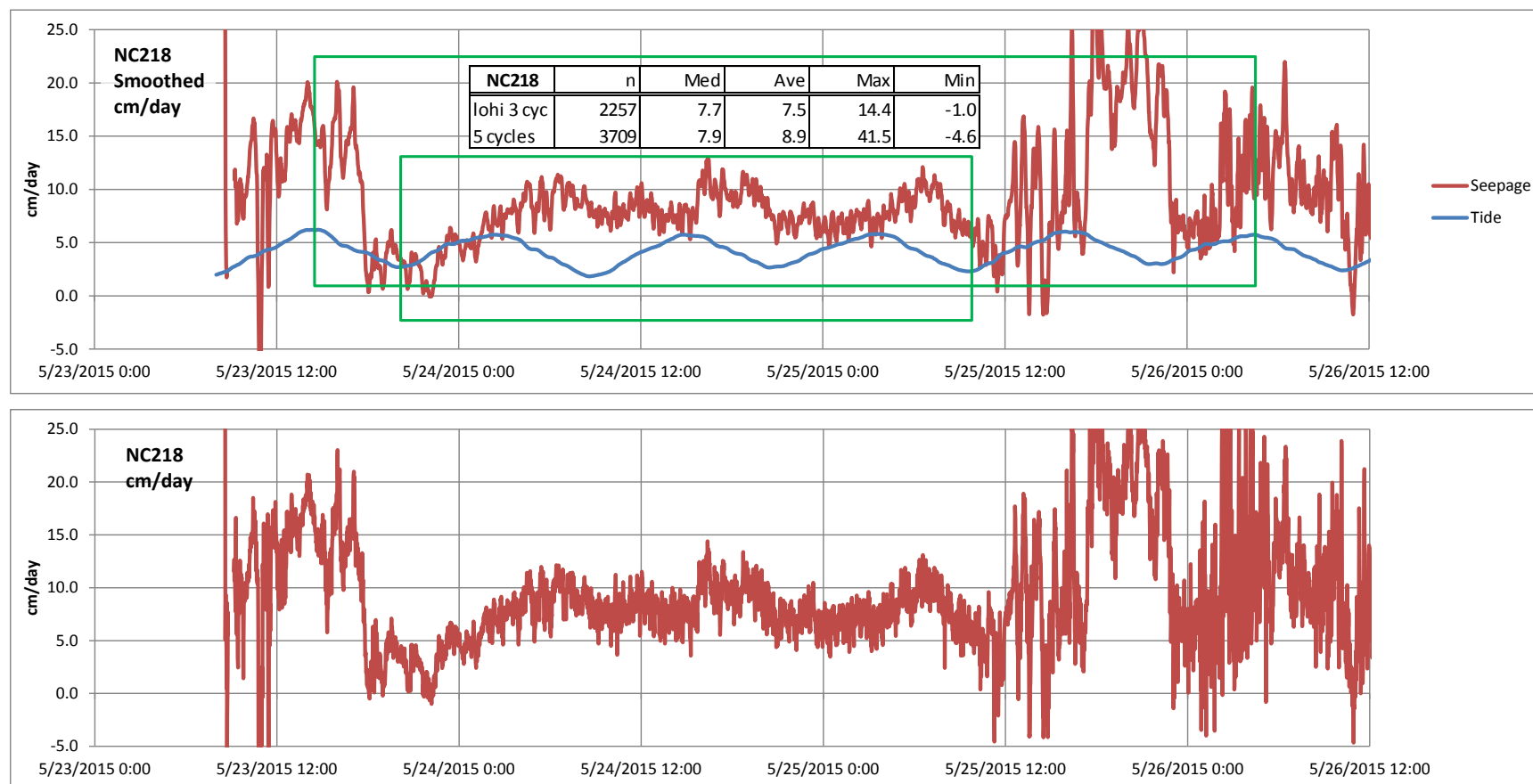
Figure 12. Seepage measured each minute during deployment at NC218, in centimeters per day. The upper plot displays smoothed data based on a 7-minute moving average, and relative tide, in feet. The lower plot presents the actual 1-minute values. The green rectangles indicate the duration of the data-summary periods. In the inset table, “lo hi” indicates one complete tidal cycle beginning and ending with low tide, and “3 cyc” and “5 cycles” indicate the number of tidal cycles during which seepage was measured. (cm/d, centimeters per day; n, number of 1-minute values; Med, median of n values; Ave, average of n values; Max, maximum of n values; Min, minimum of n values; cyc, cycles)
