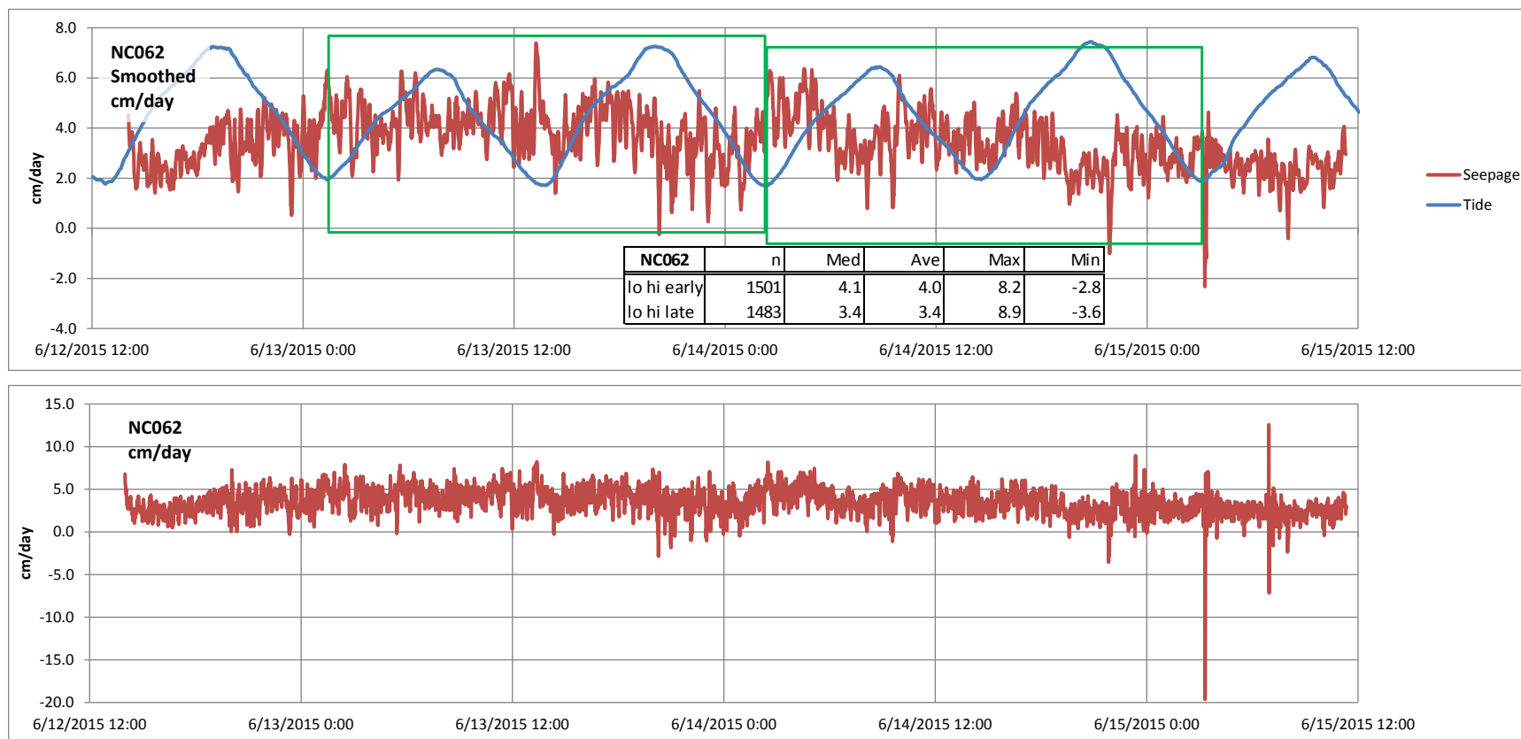
Figure 25. Seepage measured each minute during deployment at NC062, in centimeters per day. The upper plot displays smoothed data based on a 7-minute moving average, with relative tide, in feet, plotted on the right axis. The lower plot presents the actual 1-minute values. The green rectangles indicate the duration of the data-summary periods. In the inset table, “lo hi” indicates one complete tidal cycle beginning and ending with low tide, and “early” or “late” indicates timing of an analysis period relative to the site-specific data-collection period. (cm/d, centimeters per day; n, number of 1-minute values; Med, median of n values; Ave, average of n values; Max, maximum of n values; Min, minimum of n values)
