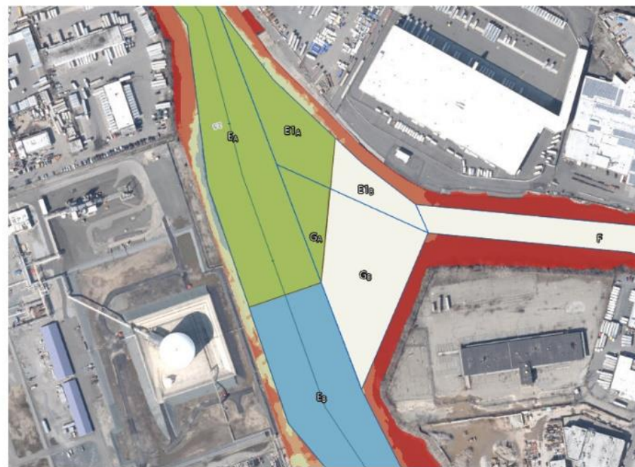
Turning Basin size reduced (portions of Reach E1 and G can be deauthorized) based on discussions with Tug Operators
