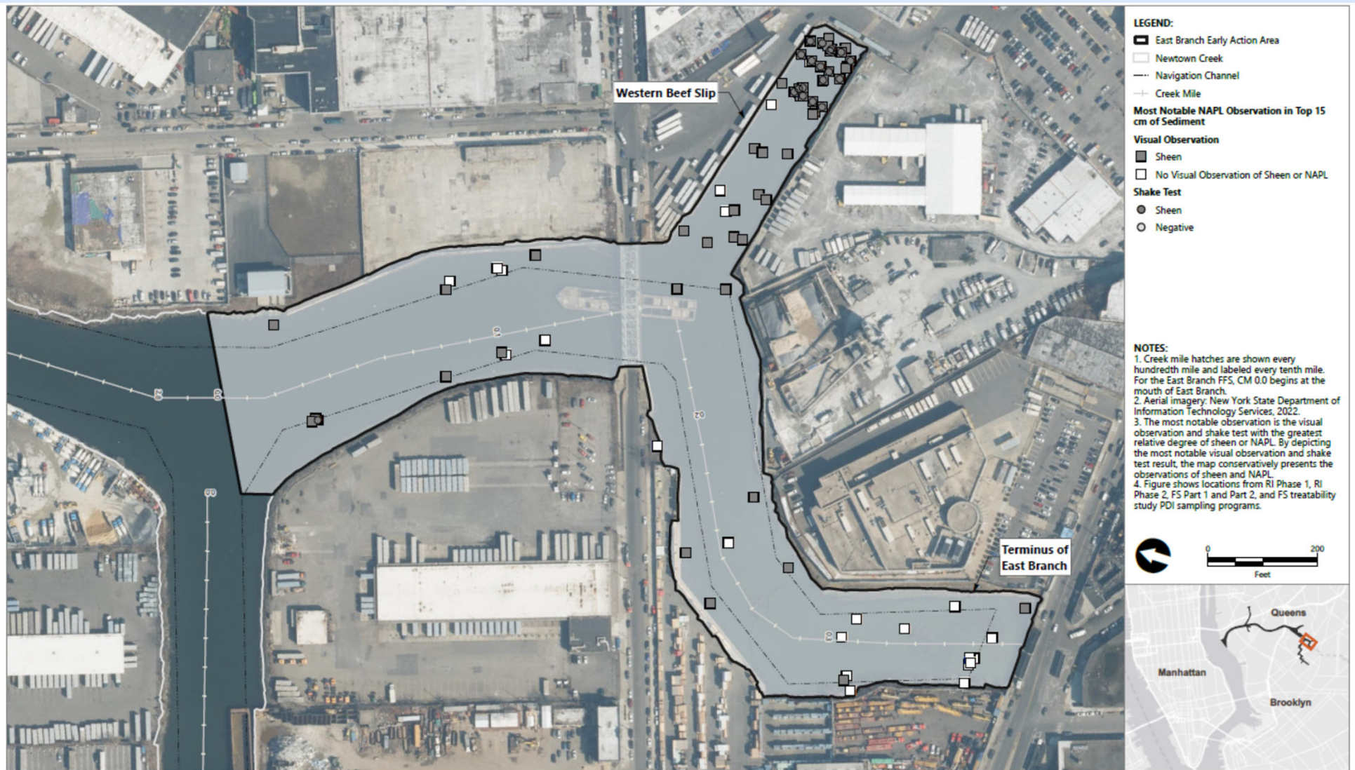
Figure A2-10a Most Notable NAPL Observations in Surface Sediment Conceptual Site Model Newtown Creek RI/FS
