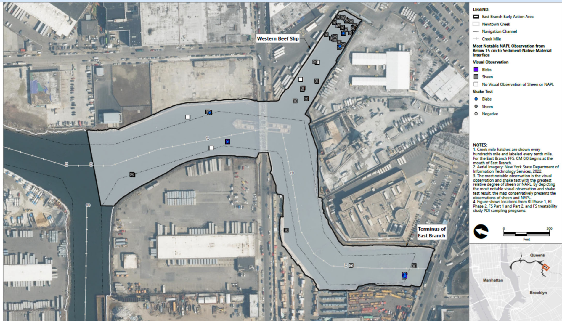
Figure A2-10b Most Notable NAPL Observations in Subsurface Sediment Conceptual Site Model Newtown Creek RI/FS
