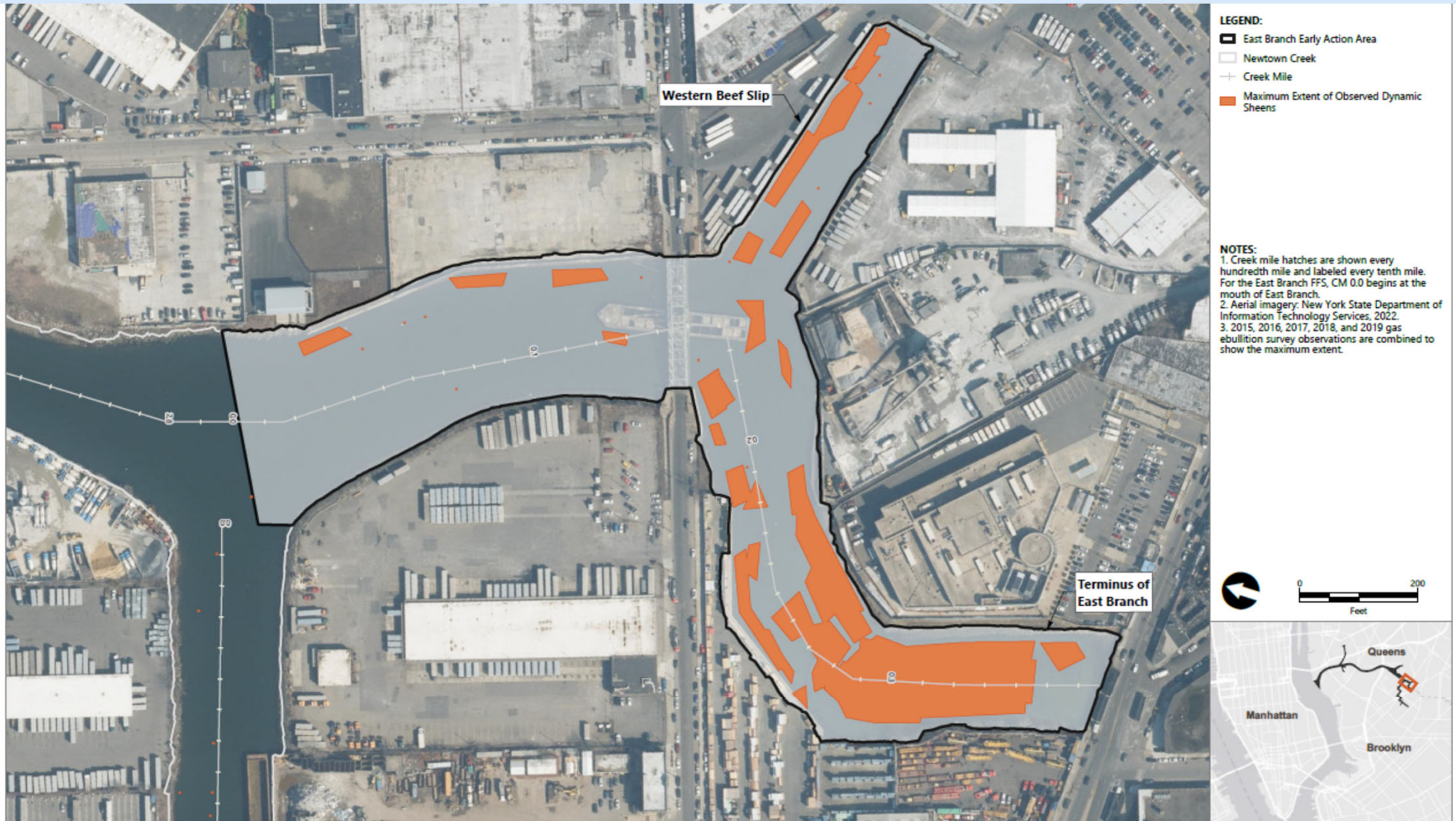
Figure A2-16 Maximum Spatial Extent of Gas Ebullition Associated Dynamic Sheens Conceptual Site Model Newtown Creek R/FS
