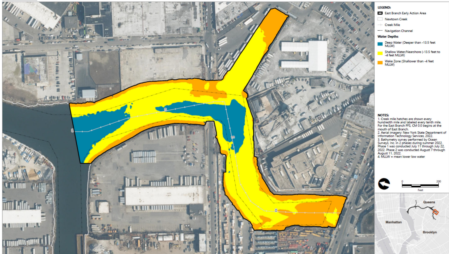
Figure 5-8 Water Depth Zones for Capping Evaluations East Branch Early Action Focused Feasibility Study Newtown Creek RI/FS
