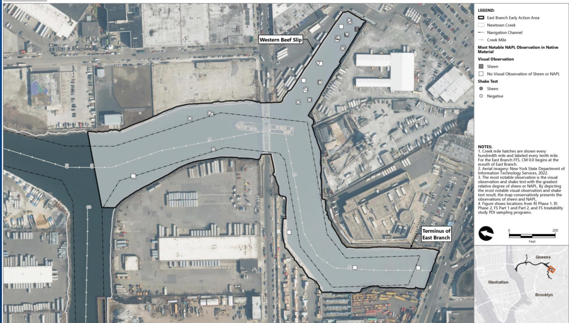
Figure A2-10c Most Notable NAPL Observations in Native Material Conceptual Site Model Newtown Creek RI/FS
