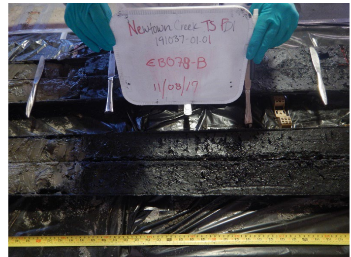
NAPL blebs observed on core from 2019 Treatability Study in the East Branch. Blebs typically not visible in photos and are confirmed with shake test.
