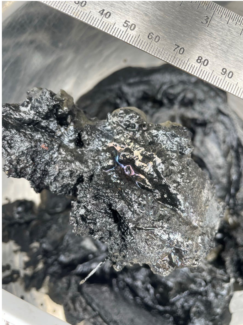
Sheen in surface soil sample collected from turning basin during 2024 FS SDC.
